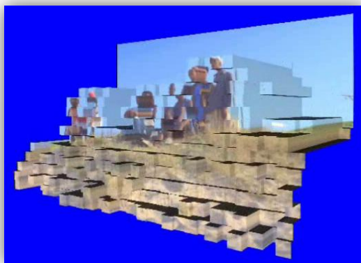
Figure 3 : Depthsafe Pinboard View at 32x18 resolution, with original video texture blown on. (“Wild Ocean” material used with kind permission ©Copyright Yes/No Productions Ltd and Giant Screen Films 2010)
